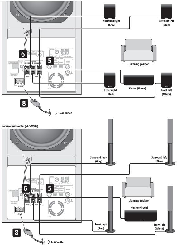
• Connect the other end to the color-coded speaker terminals on the rear of the receiver subwoofer. Make sure to insert completely.
